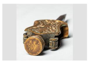
Small, flat object with a pointed end. It is a sliding scribing punch for circular arcs.
